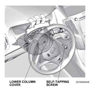
6. Turn the steering wheel 180° counterclockwise, and remove the other self-tapping screw from the lower column cover.
