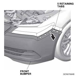
• Release the five retaining tabs on each side.
