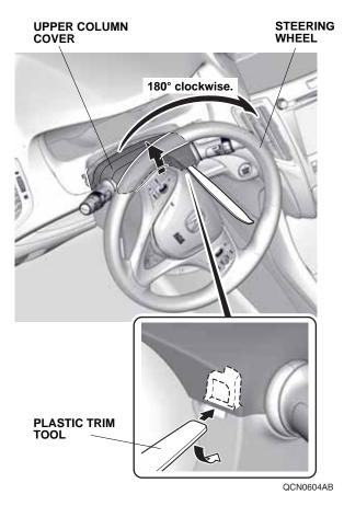
4. Pull the upper column cover upward, and secure it to the dashboard with tape.
