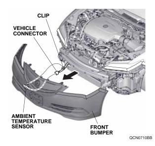
20. Remove the ambient temperature sensor.
