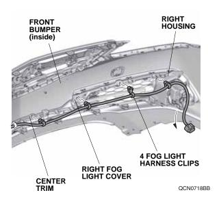
Plug the two fog light harness 3-pin connectors into the left and right fog lights.
