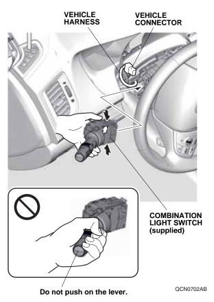
12. Plug the vehicle connector into the new light switch. Make sure the vehicle harness is not being stretched. 13. Attach masking tape to the front bumper, headlights, and front fenders as shown.
