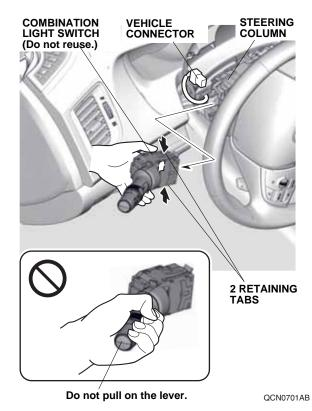
10. Push in on the two retaining tabs, slide the light switch out, and remove it from the steering column. Do not pull on the lever.
