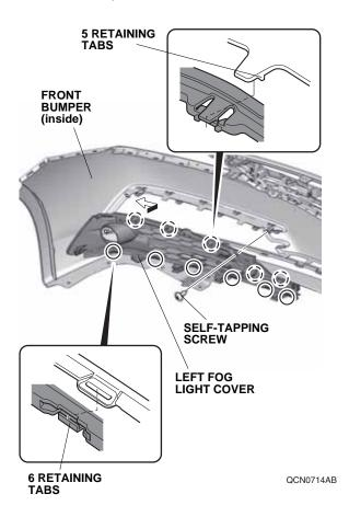
25. Secure the left housing with one self-tapping screw, two self-tapping screws removed in step 23, and one clip.
