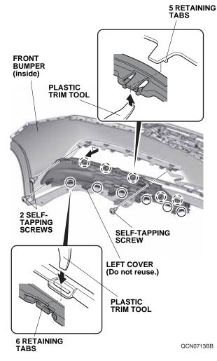
24. Secure the left fog light cover to the front bumper with eleven retaining tabs and the self-tapping screw
