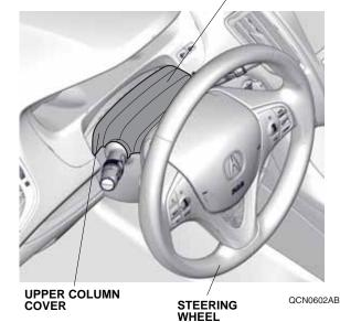
2. Press the engine switch to ON. Turn the steering wheel 90° counterclockwise. Using a plastic trim tool, release the upper column cover.
